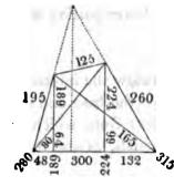
Length of the base 300. Summit 125. Flanks 260 and 195. Diagonals 280 and 315. Perpendiculars 189 and 224.
