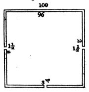
Here the area of the exterior figure is 10,000: that of the interior one 9216. The difference is 784. It is the area of the figure covered by the walls. Multiplied by the height 7, it gives the content 5488; from which subtracting the gates 36, the remainder is the exact cubic content 5452. Dividing this by the content of a brick 18, the quotient is the number of bricks 65424.
