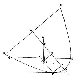
Let the plane through AM perpendicular to the surface of the fluid cut the paraboloid in the parabola BAB' and the plane of the surface of the fluid in QQ'. Let PT be the tangent parallel to QQ', PV the diameter bisecting QQ'. Divide AM at C, O as before, and draw OL perpendicular to PV.
