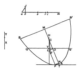
Let X + Y be a straight line such that (spec. gr. of solid) : (spec. gr. of fluid) =  $(X + Y)^2$  :  $am^2$ .....( $\alpha$ ), and suppose X = 2Y.
