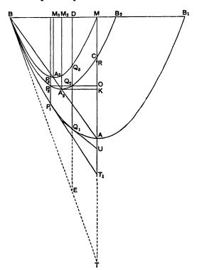
On  $A_2M_2$ ,  $A_3M_3$  as axes describe parabolic segments similar to the segment  $BAB_1$ . (It follows, by similar triangles, that BM will be the base of the segment whose axis is  $A_3M_3$  and  $BB_2$  the base of that whose axis is  $A_2M_2$ , where  $BB_2 = 2BM_2$ .)
