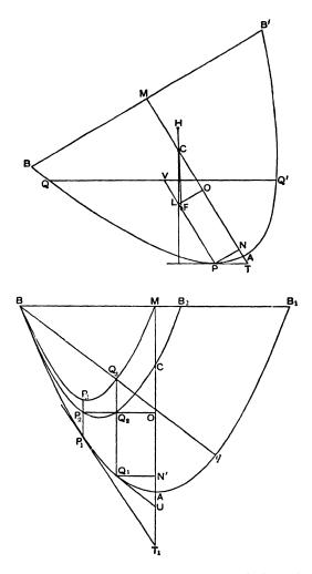
plane of the surface of the fluid in QQ'. Let PT be the tangent parallel to QQ', PV the diameter bisecting QQ', PN the ordinate at P.
