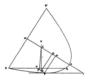
Let the plane through AM perpendicular to the surface of the fluid cut the paraboloid in the parabolic section BAB'and the plane of the surface of the fluid in BQ.
